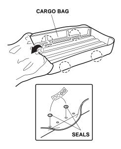
4. Using isopropyl alcohol on a shop towel, thoroughly clean the area where the large pad will attach.
