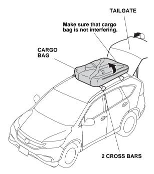
2. With the help of an assistant, carefully unfold the cargo bag on the cross bars.
