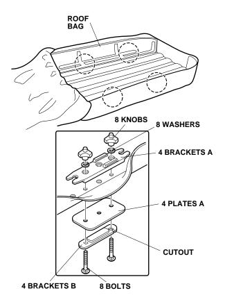
11. Loosely install bracket A, four plates A, and bracket B to the cargo bag with two bolts, two washers, and two knobs for each location shown. Be sure the cutout on bracket B is facing outward.
